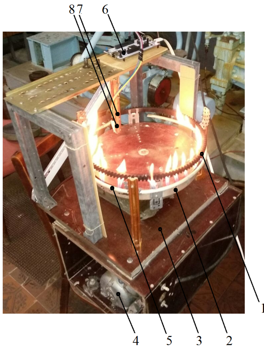
Figure 10 – General view of the heating installation: 1 – model of the gear ring; 2 – rotary platform; 3 – installation casing; 4 – electric drive; 5 – gas burner; 6 – measuring equipment; 7 – temperature sensor; 8 – distance sensor
